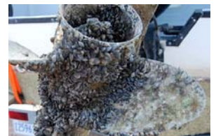
Zebra mussels covering the lower unit of a motor.
